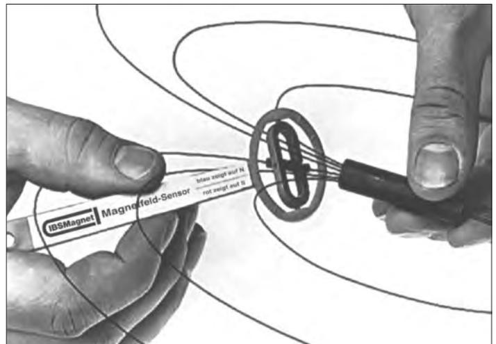
A small magnet and the needle of a compass follow the magnetic flux lines. (IBS Magnet field sensor Type MK II)
