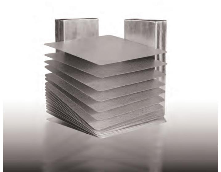
Stacked steel plates can be separated with spreading magnets. As shown above the separation of plates can be done by different arrangements of the spreading magnets at the pile of sheets. Only steel with magnetic conductivity can be separated.
